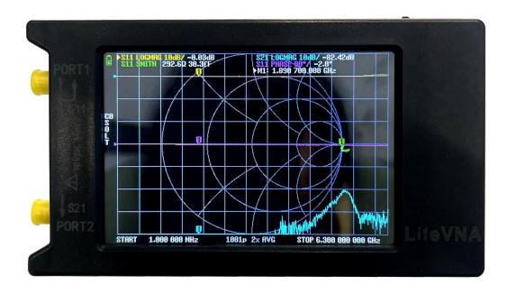
Figure 1: The LiteVNA 64 with a range of 50 kHz to 6.3 GHz.
